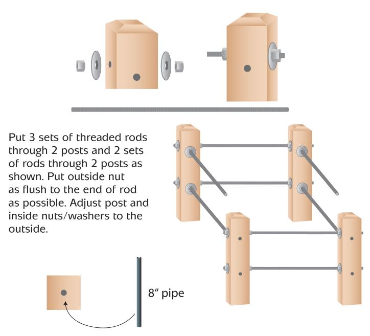
Turn both sides upside down and hammer the four 8" pipes into the bottom insets.
